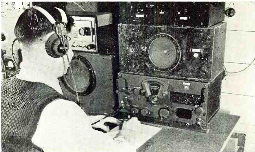
You can copy weak signals through interference much more readily with a pair of phones than with a loudspeaker. Besides, the high-pitched dits and dahs from the latter can be most annoying to other members of the household.
