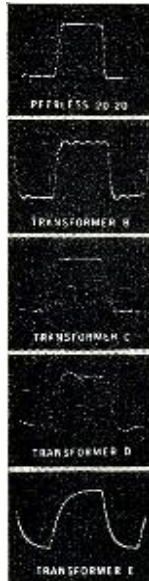
Photos show square wave response with 11,000 cycle fundamental frequency
